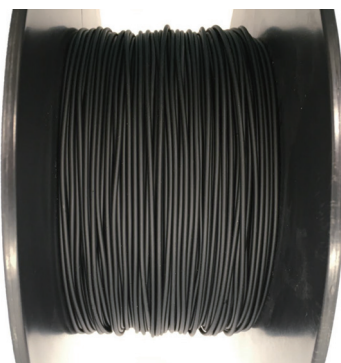
图8 RGO/PLA复合材料3D打印丝材 Fig.8 RGO/PLA composite filament for 3D printing
